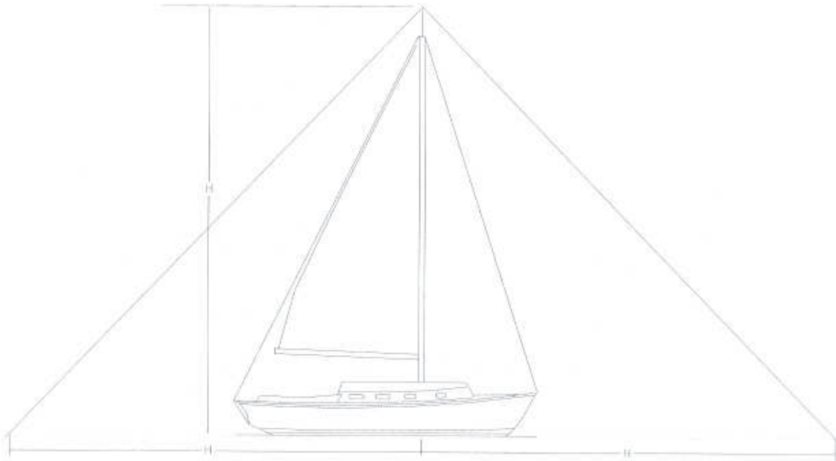
FIGURE 1 – ZONE OF PROTECTION BOAT WITH MAST NOT EXCEEDING 100 FEET ( 30 M) ABOVE THE WATER
